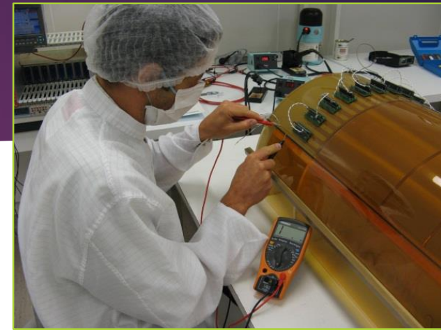
Electric leak test
