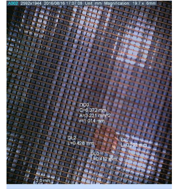
Shadows of the area irradiated at 200kHz/mm 2 on a readout plate
