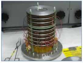
existing chamber up to 10 actinide targets measured simultaneously
