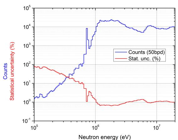
High statistics and resolution cross section data > 600 keV (investigation of resonant structure at threshold + data up to high energies)
