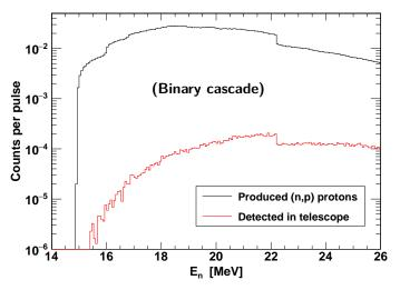
Detected counts reduced due to the limited solid angle, i.e. the geometrical efficiency. (discontinuities: an artifact of the Binary cascade, selected purely for the integral yield closest to the n\_TOF value)
