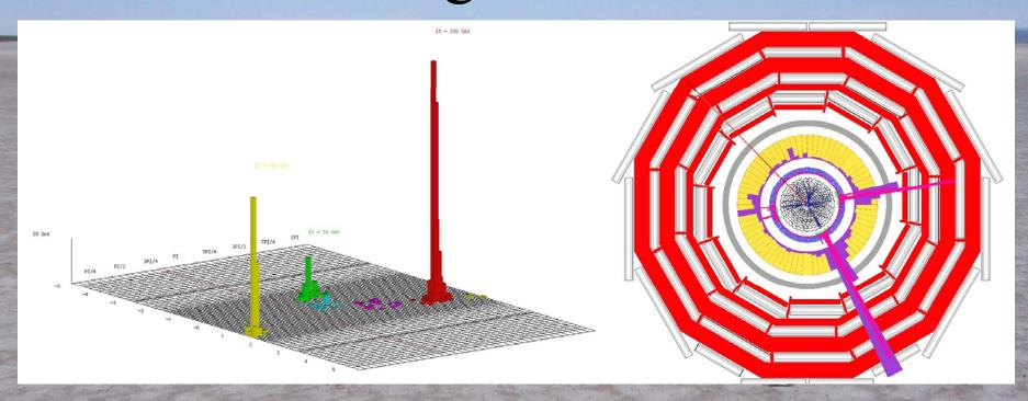
Missing transverse energy carried away by dark matter particles
