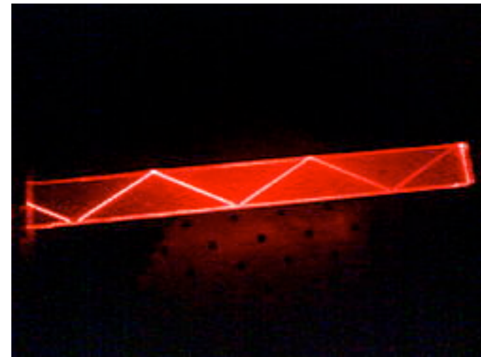
Total internal reflection in a block of PMMA
