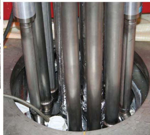
The cryogenic chimney links the cold mass to the phase separator cryostat by SDMS (F)
