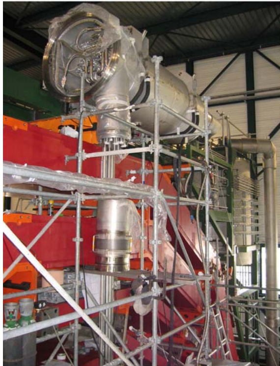
The cryogenic chimney links the cold mass to the phase separator cryostat by SDMS (F)
