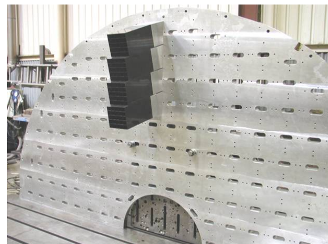
Dee backplate with 4 supercrystals
