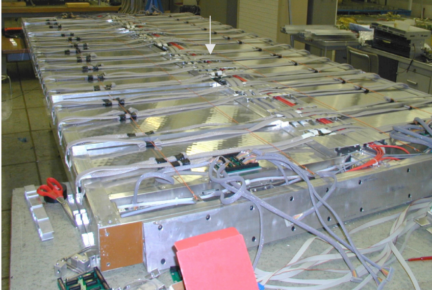
RPC preassembly & cabling
