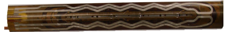
Photo: Protection heaters in LARP Nb3SN HQ quadrupole.
