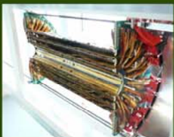
Above—1/2 of CMS barrel pixel detector Below— Conceptual design of new readout for upgraded pixel detector
