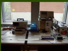
Above—test setup for micro twisted pair wire testing
