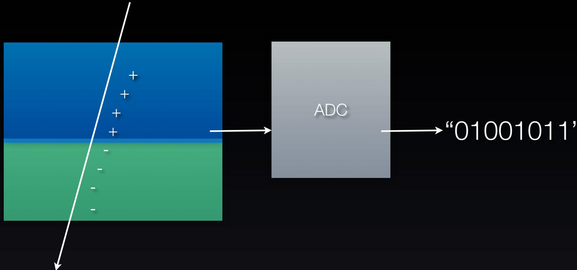
○○○ Charged Particle Ionizes Silicon
