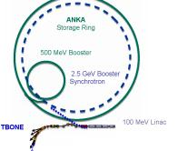
TBONE could also be used as the first stage of a full energy injector to the existing ANKA storage ring.
