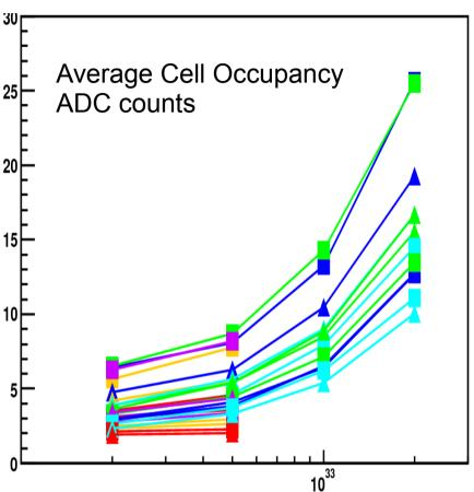
Signal in 12 cells on the ECAL surface Min-bias events (Gauss)
