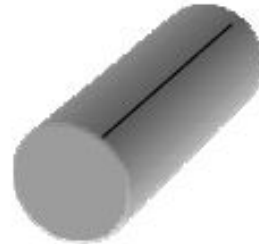
Rolled tube & longitudinal weld (EB)
