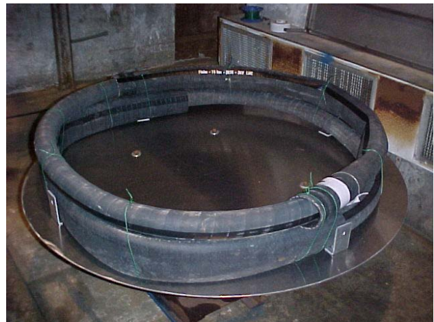
Figure 11: Total Dose Irradiation of cables for the powering of the inner triplet magnets of the LHC.
