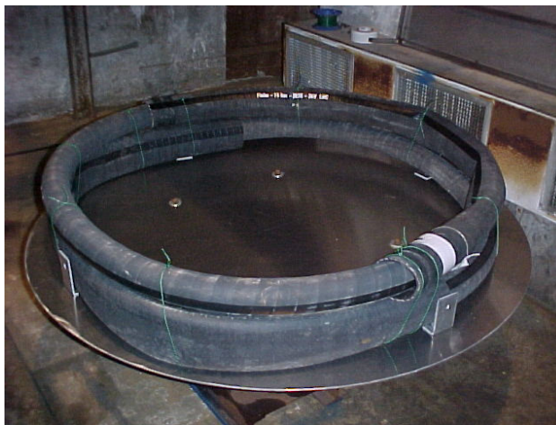
Figure 11: Total Dose Irradiation of cables for the powering of the inner triplet magnets of the LHC.
