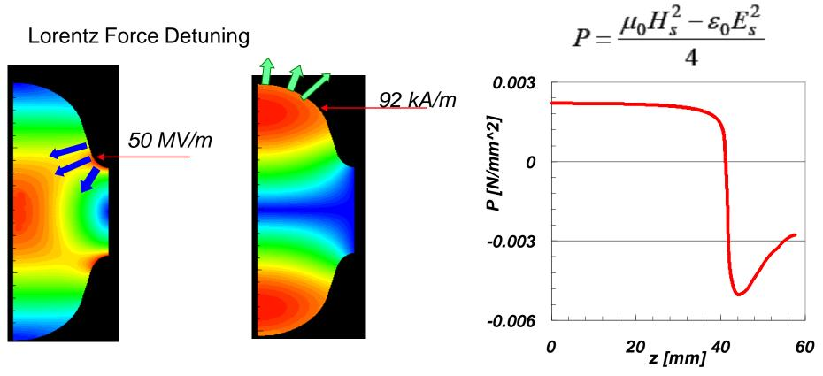
E and H at  $E_{acc} = 25 MV/m$  in TESLA inner-cup
