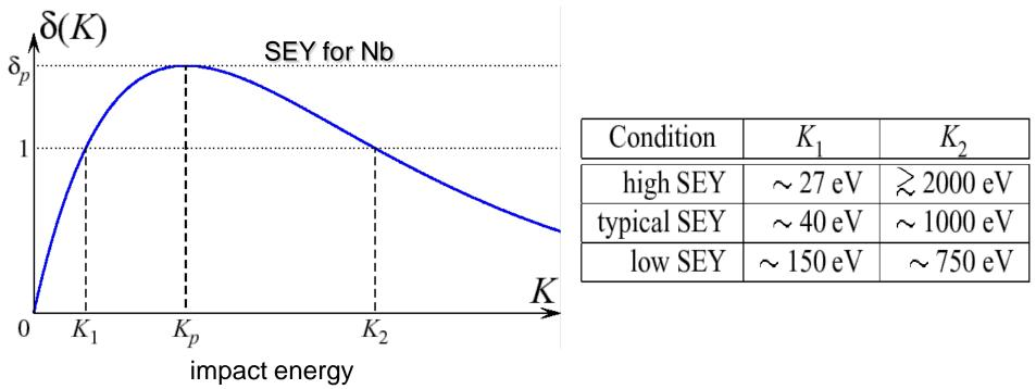
When happens, multipacting is barrier in rising the accelerating field in cavities and usually leads to quench.
