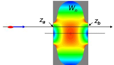
Trajectory of the point charge q, assumed here is a straight line.
