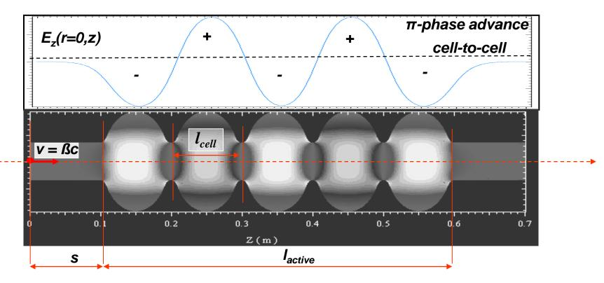
Synchronic acceleration and max of  $(R/Q)_{acc}$  for a multi-cell structure when:
