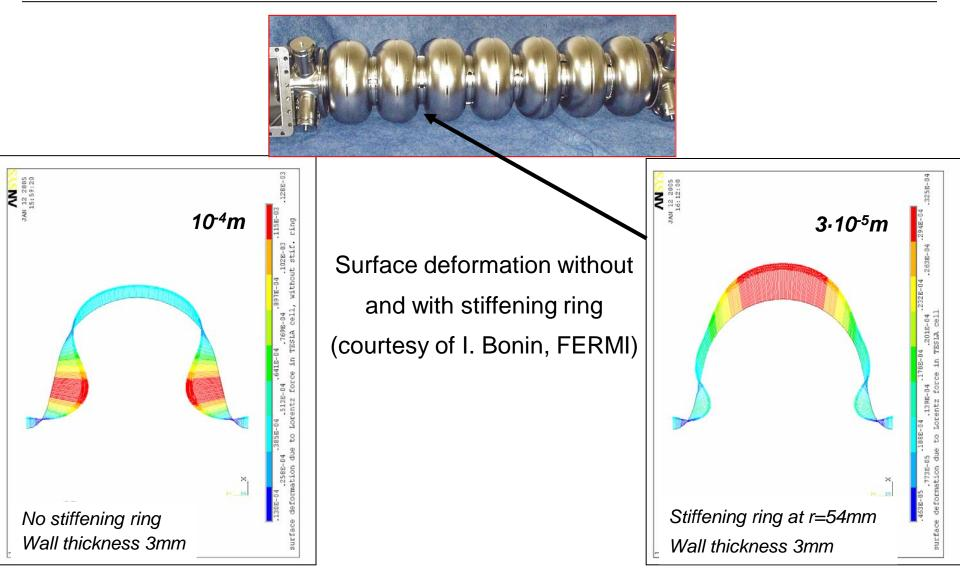
Essential for the operation of a pulsed accelerator  $\Delta f = k_L (E_{acc})^2$   $k_L = -1 Hz/(MV/m)^2$
