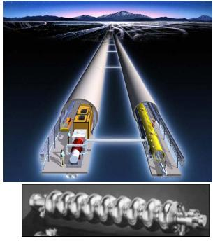
$E_{acc}$  > 34 MV/m shown in several 9-cells in the cw test.
