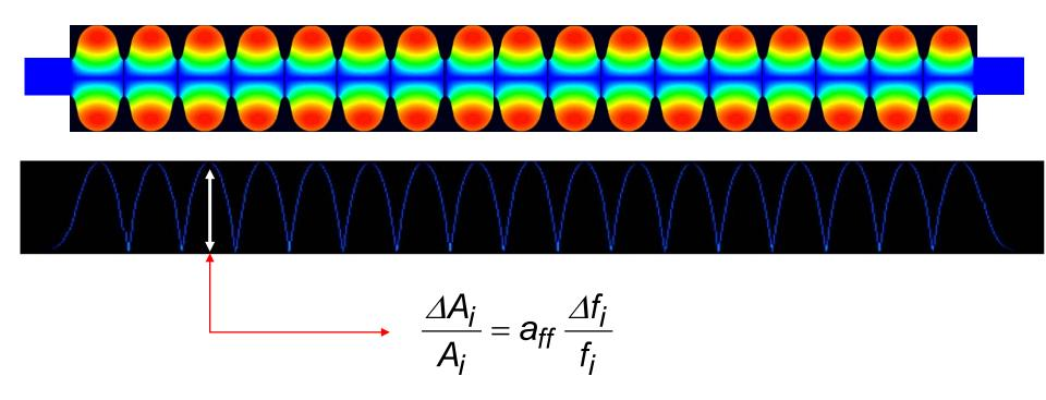
Field flatness factor  $a_{ff}$  for structure made of N cells and their coupling factor  $k_{cc}$
