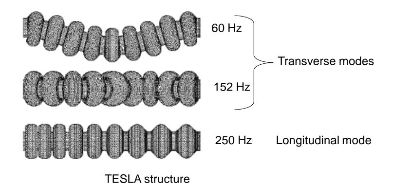
The mechanical resonances modulate frequency of the accelerating mode. Sources of their excitation: vacuum pumps, ground vibrations...
