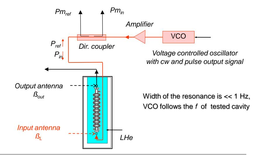
At first, in these tests one measures the coupling strength  $\beta_L$  and  $\beta_{out}$  of the input and output antennae.
