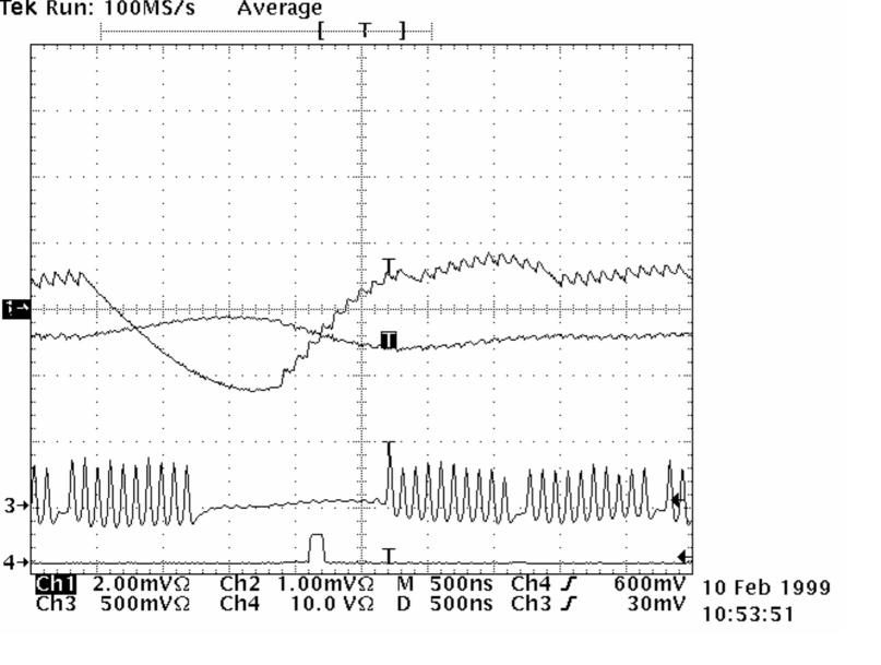
Transient behaviour of the cavity voltage under the influence of fast feedback. (Courtesy of Elmar Vogel [9])
