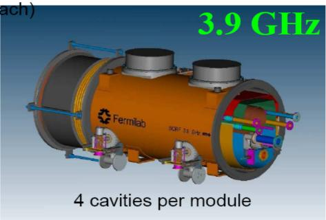
TESLA type cavities have been scaled down in size to fit the 3.9 GHz. All auxiliaries like coupler, HOM coupler, frequency tuner, etc..., are scaled as well. Most of this work was done by H.Edwards et al. / FNAL.
