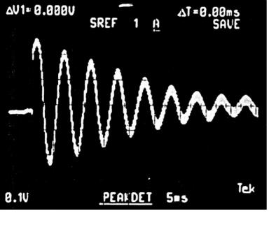
The synchrotron oscillation measured at the phase detector output a few ms after injection of a batch of 9 proton bunches into PETRA II. It is smeared out by Landau damping after some periods. The damping loop is not active.
