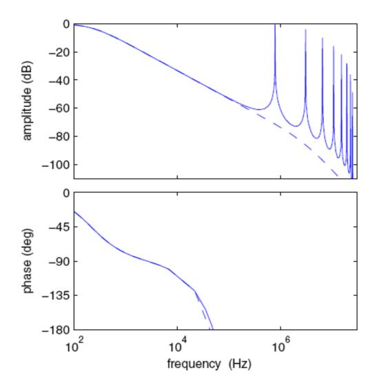
FIG. 4. (Color) Bode plot of the continuous single cavity open loop transfer function (7) with unity gain (G = 1) and loop delay  $\tau_{\text{loop}} = 5 \ \mu \text{s}$ . At the dashed line all FMs with exception of the  $\pi$ -mode have been omitted.
