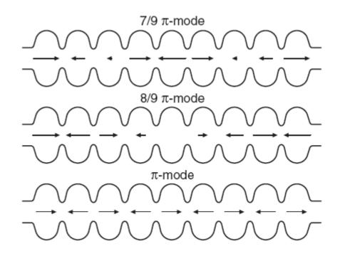
FIG. 2. The rf field amplitudes of the normal and fundamenta modes (FMs) in 9-cell cavities.
