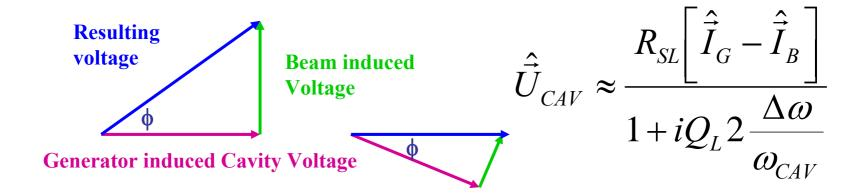
In the case of pure reactive beamloading, i.e. when  $U_{CAV}$  and  $U_{B}$  are in quadrature, the original cavity voltage can be restored by detuning the cavity. No additional generator power is needed in steady state, but for transient beamloading compensation sigificantly more power may be needed.
