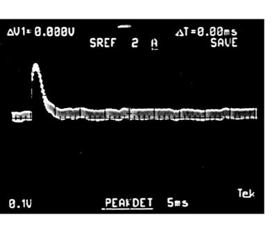
Here the phase loop is active. The synchrotron oscillation is completely damped within half a synchrotron period of 5 ms.
