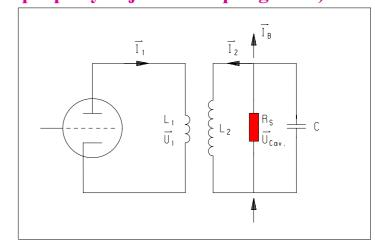
$$\omega_{CAV}^{2} \vec{U}_{CAV} = \frac{1}{C} \left[ \frac{1}{N} \dot{\vec{I}}_{1} - \dot{\vec{I}}_{B} - \frac{1}{R_{S}} \dot{\vec{U}}_{CAV} \right] - \ddot{\vec{U}}_{CAV}$$
