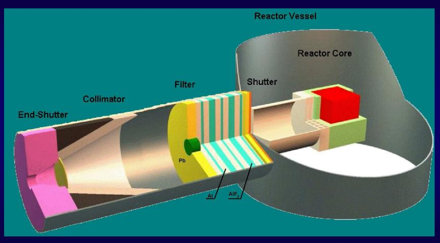
Online epithermal/fast neutron flux monitoring performed with fission chambers ( $U^{235/238}$ ) inside the collimator
