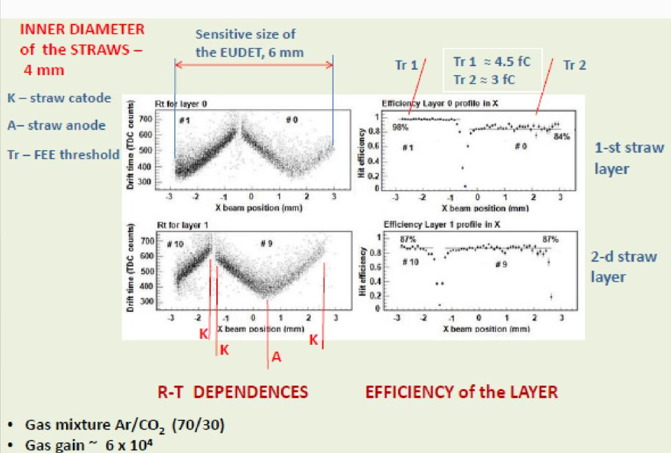
Typical Spatial Resolution (~ 180 μm) and Efficiency (≤99%)
