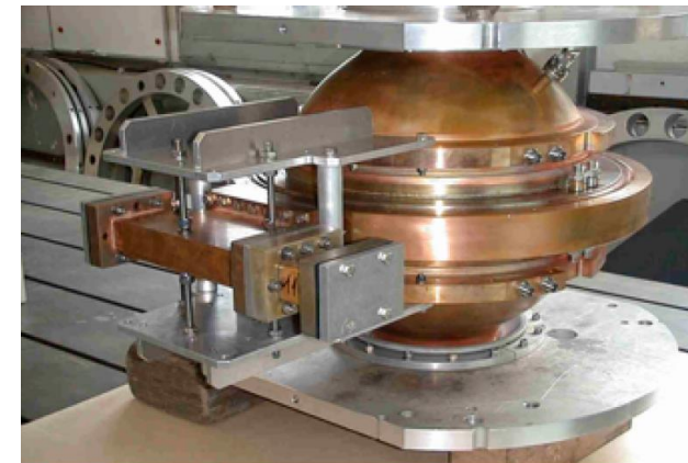
Fig. 3.2.4.11: 3 GHz BOC used at the CLIC Test Facility (CERN).
