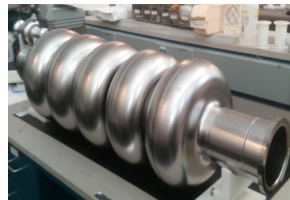
prototype FCC 5-cell 800-MHz Nb cavity (at JLAB, 2017)
