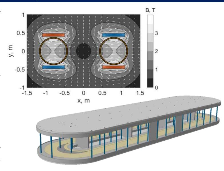
Design shows two racetrack coils in quadrupole layout, allowing for 2 free bore tubes of Ø 700 mm.
