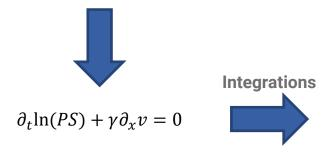
$$P(t) = P(0) \left(\frac{V(0)}{V(t)}\right)^{\gamma} \exp\left(\gamma \int_{0}^{t} \frac{q_{v_0} - q_{v_L}}{V(t)} dt\right)$$
