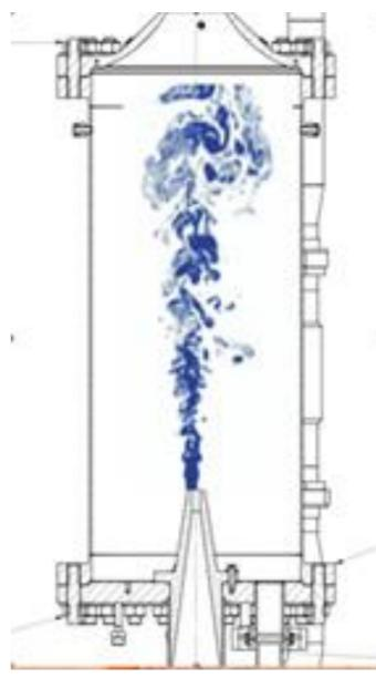
The jet is generated by the expansion of the liquid helium which is set in movement by a rotating pump, and cooled via a copper heat exchanger
