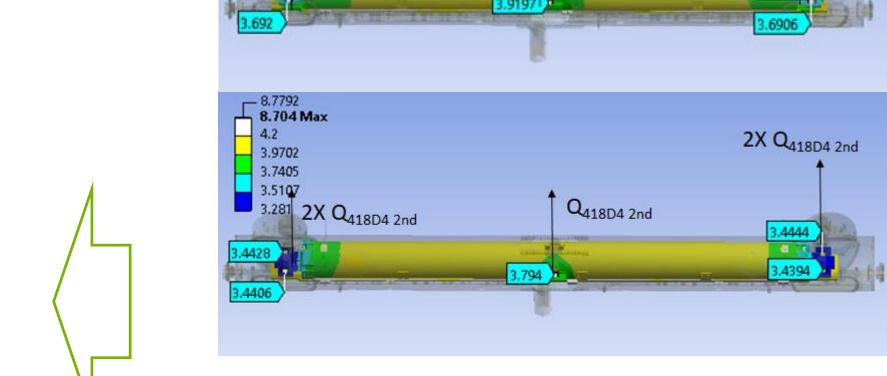
head are higher, however, the total cooling powers are lower than using 418D4's By using Five 418D4s, the cold head temperature 3.4K and 3.8K yields total 5.61 W of the cooling power. LHe tank is maintained at 4.2K. additional
