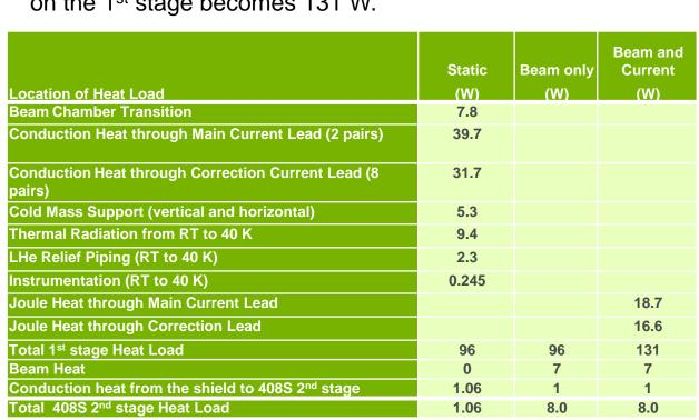
The original design with 415D has excess cooling
