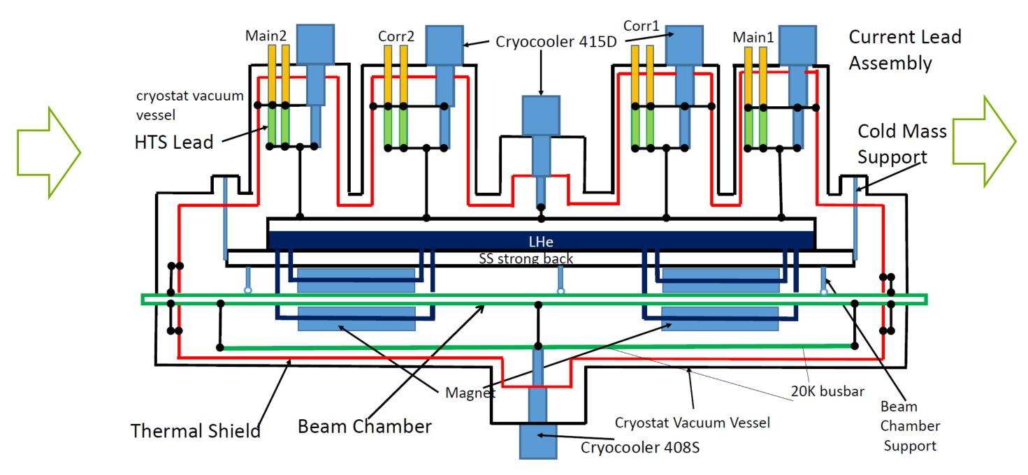
The APSU-SCU cryostat is a one shield cryostat (similar to the 2<sup>nd</sup> generation cryostat) but with three thermal circuits.
