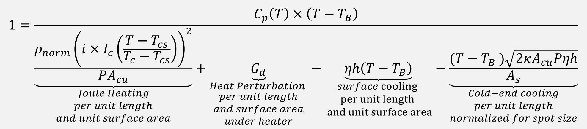
•  $C_p$  calculated from experimental data fit from PPMS data from Nb<sub>3</sub>Sn strand at 12 T [3]
