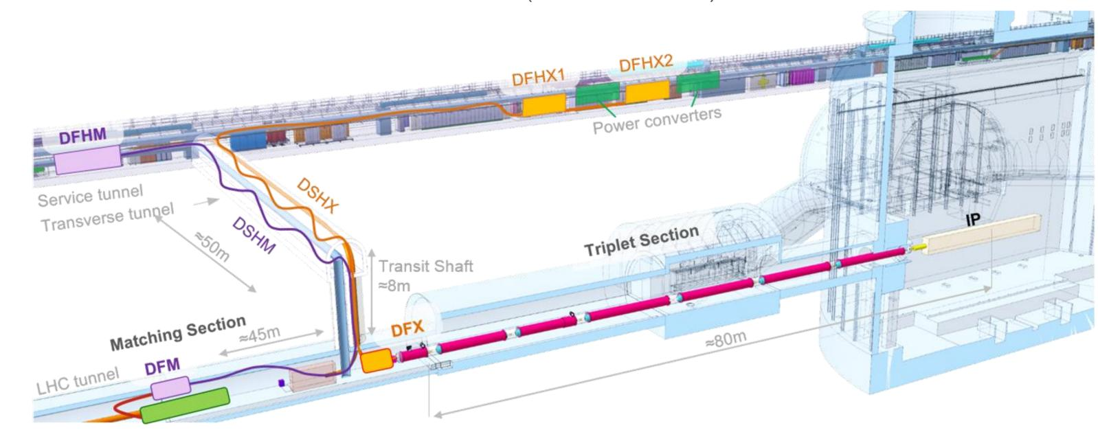
Warm cables connect the Power converters to the current leads 300K side. HTS cables connect the current leads to the MgB<sub>2</sub> cables in the DFH. In the DFX, the MgB<sub>2</sub> leads present NbTi extensions, connected to the  $\lambda$  plate's leads.
