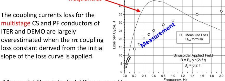
P. Bruzzone et al. "A new test method of AC loss assessment for fusion conductors", Fusion Eng. Des. 146, 2019, pp. 928-931.
