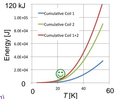
Energy needed to heat the 32 T HTS windings (~80 kg)
