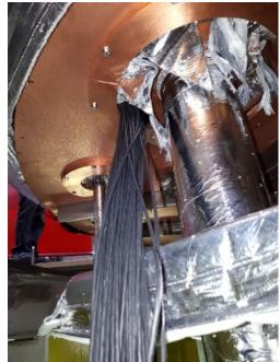
Feedthrough for the 212 instr. wires (vacuum side)
