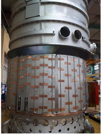
Trial assembly in industry of the OVC with thermal shields
