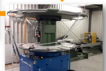
Winding the 1<sup>st</sup> layer after having stored on the upper part the conductor length for the 2<sup>nd</sup> layer
