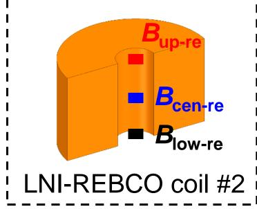
Magnetic fields homogeneously decayed in the axial direction.
