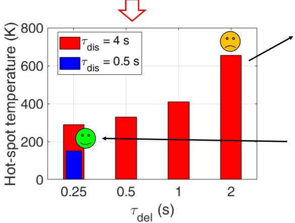
Same τ<sub>dis</sub> for CS and insert → too high hotspot temperature
