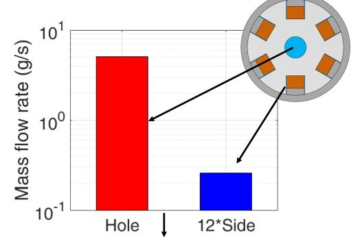
Total dm/dt in side channels ~ 1/20 dm/dt in hole
