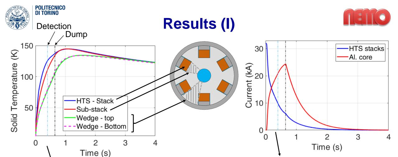
Temperature differences between stacks and core > 40 K→ issues on thermal stresses to be addressed in the future
