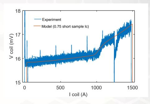
Voltage transient modelled with two tape in parallel or a single « super tape » hypothesis very close much lighter model : real time calculation ?
