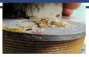
Testing this coil at 3 T and 5 T further supports the argument that the mid tap was the root cause of Pup-6's less than desired performance.
