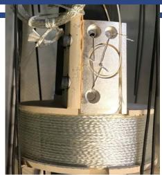
Pup-7 was to be run in a 14 T outsert. The coil was well reinforced and did not include a mid tap. The strain-limited performance limit is indicated on the right.
