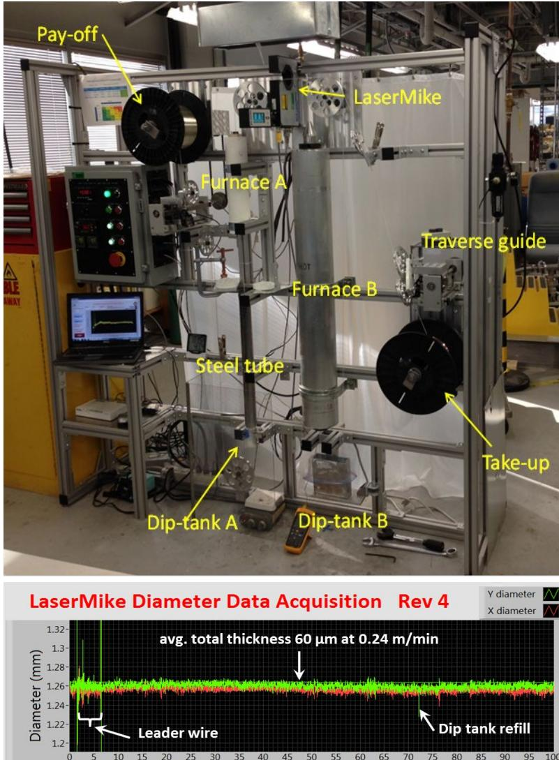
In-house insulation facility (top) and diameter measurement (bottom)
