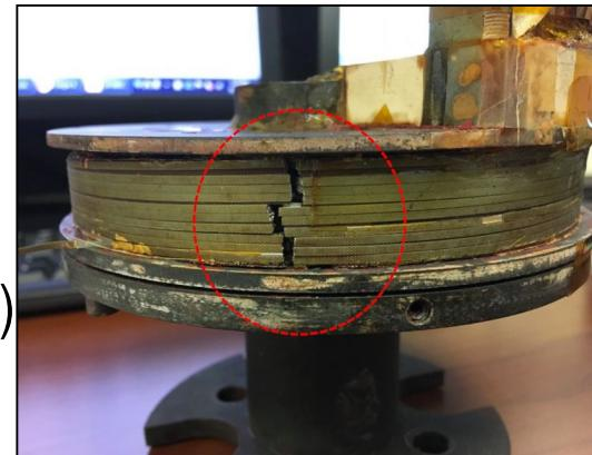
Test Coil snapped at  $\sim 175 \text{ MPa}$
