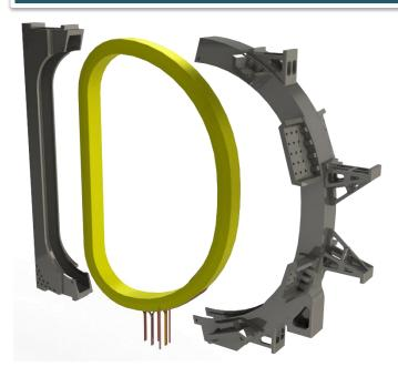
Simmetric shape of TF coils to allow DN and other possible simmetric scenarios (wrt equatorial plane). All the magnet system weight loads the TF coils. Structures are mainly based on machining of 316L(N) forged sectors.
