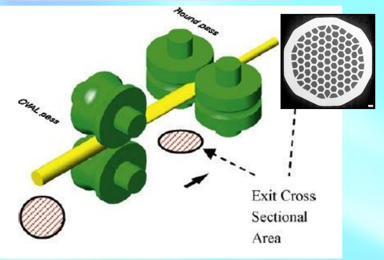
➤ Groove rolling can maintain the integrity of filament by maintaining higher Ag ratio than drawing process
