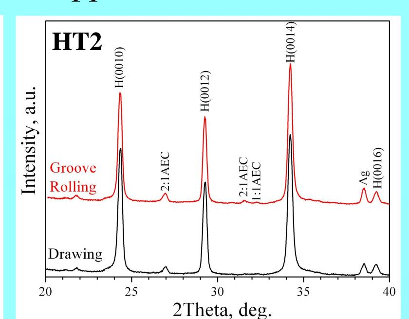
Obviously enhanced density can be observed in Groove rolled tapes.
