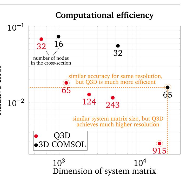
⇒ The Q3D method delivers accurate results (even better with spectral mesh adaptation) and needs much less computational effort than the conventional 3D FEM to do so.
