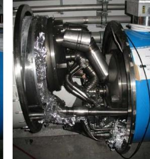
"Within the first second, an electrical arc developed and punctured the helium enclosure, leading to release of helium into the insulation vacuum of the cryostat [...]. [The resulting large pressure] forces displaced dipoles [...] and knocked the short straight section cryostats housing the quadrupoles and vacuum barriers from their external support jacks [...], in some locations breaking their anchors in the concrete floor of the tunnel."
