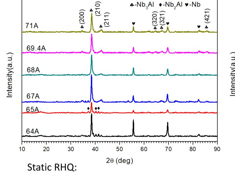
$\epsilon I_{RHO} \leq 65A$ , brittle, Nb<sub>2</sub>Al+A15 after 800 °C 10h  $\epsilon I_{RHO} = 67^{\circ}71A$ , ductile, A15 after 800 °C 10h
