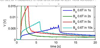
The mockup was tested in the Josefa Facility (CEA / up to 1T/s). Model (dashed) is confronted to the experimental measurements (plain) in these induced voltage curves...
