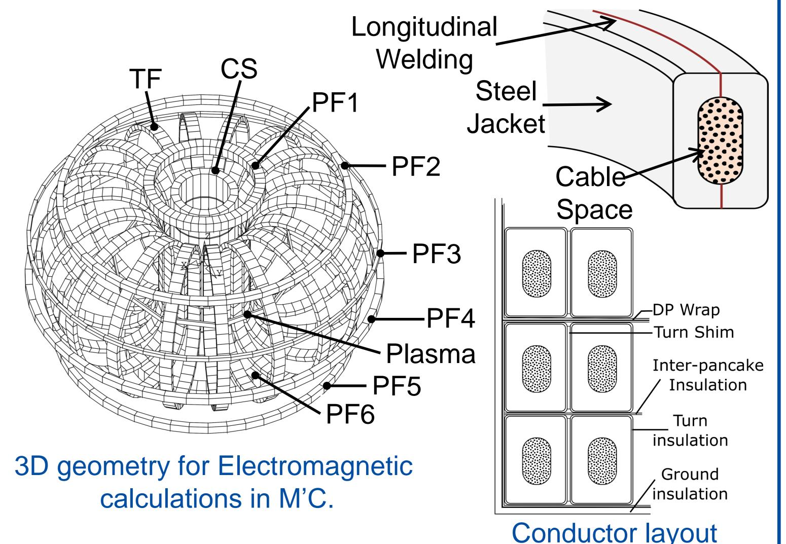
\*Plasma is modeled as rectangular cross-section coil in center: H=500mm,  $W=200mm, I_{plasma}=17.86 MA$
