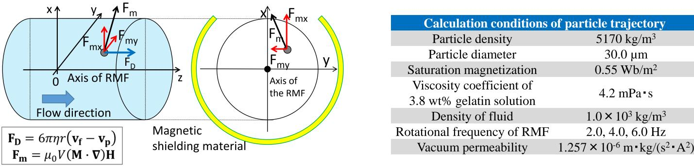
For considering the time-dependence of the magnetic field, magnetic field was calculated when the shielding material was rotated every 30 degrees. Based on these 12 magnetic field distributions, the magnetic force considering the time change was calculated. (Ansys 10.0, Cybernet System, Japan) The existence of glass beads are neglected in order to simplify the calculation system,
