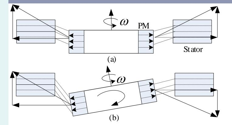
The PM rotor is passively stabilized by reluctance force in the axial and tilting directions.
