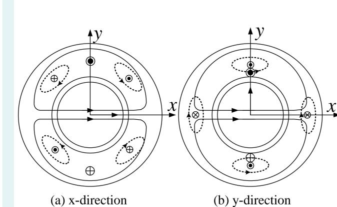
As a function of the two magnetic fields with different numbers of pole pairs, the original balanced air-gap magnetic field is broken and in this case a radial suspension force can be generated to realize the rotor stabilization. As shown in (a), the flux density in x-axis positive direction is strengthened and by contrast, that in x-axis negetive direction is weakened. Thus, a suspension force component *F* is generated in the x-direction.
