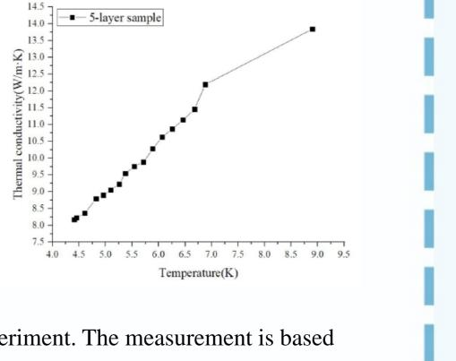
The purpose is for current lead applications, the axial thermal conductivity of soldered stacked YBCO conductors is tested by experimental platform based on a GM cryocooler. Fig.5a shows the experiment. The measurement is based on the one-dimensional Fourier heat transfer law:
