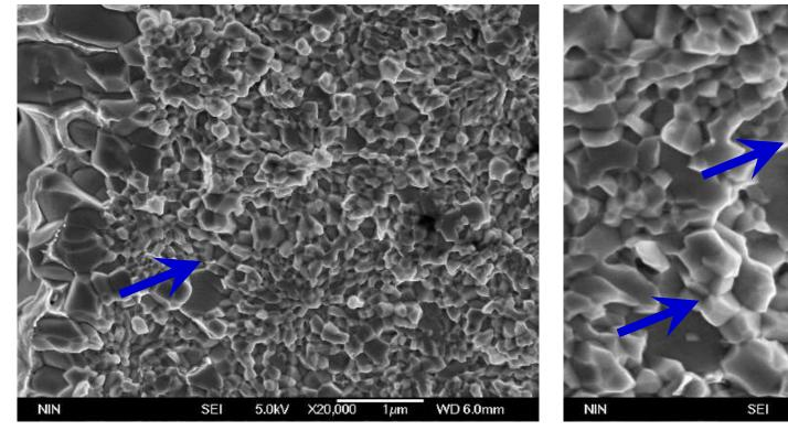
2122A/mm<sup>2</sup>@4.2K, 12T (with 300~400nm coarse grains)
