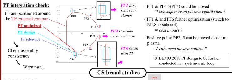
**DEMO 2015 CS:** assess the sensitivity of CS design to selected inputs
