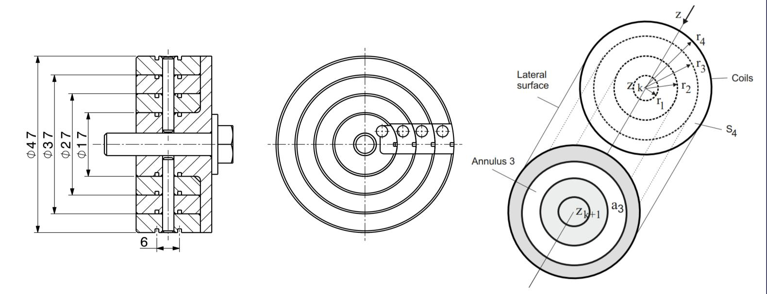
The coil surfaces  $S_i$ , are **calibrated in a reference dipole magnet**. The coil resistances are used to correct the different attenuation on the input impedance of the integrator cards. The effective coil radii  $r_i$  are retrieved from the calibrated surfaces by  $r_i = \sqrt{S_i}/(\pi N)$ , where N is the number of turns in each coil (N = 120).
