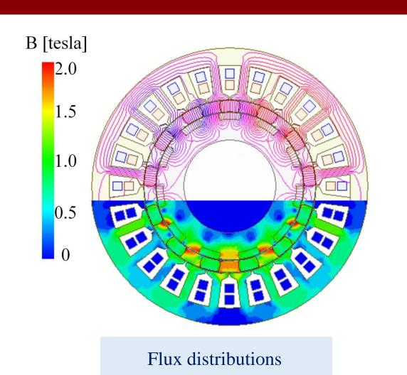
The distribution of magnetic field is calculated to verify the correctness of the theoretical analysis.
