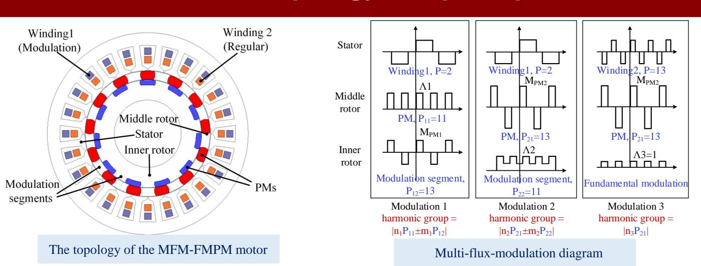
The MFM-FMPM motor consists of a stator and two internal concentric rotors, which can be regarded as the combination of three modulation motors. With the introduction of double layer PMs and two sets of windings, the motor structure is relatively compact.
