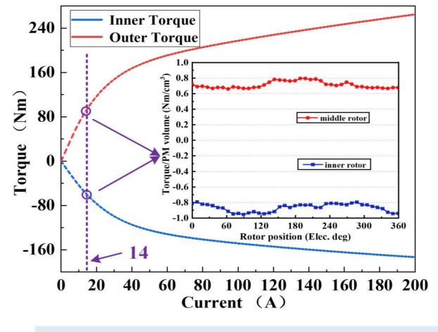
Torque-current characteristic and torque in per unit PM volume
