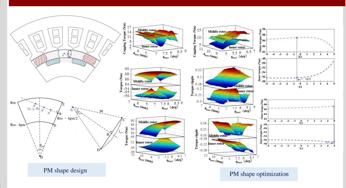
Since the PMs and modulation segments are placed adjacent, the PMs in the middle rotor and inner rotor are convex, while the modulating segments in the two rotors are concave and share the same arc with the PMs.
