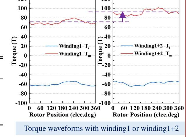
In order to display the improvement in torque density, two cases are modeled for comparative study: motor with single layer PM (PMs in the inner rotor or middle rotor) or with double layer PMs (PMs in the inner rotor and middle rotor) (case 1), and motor only with modulation winding(winding1) or added with regular winding(winding1+2) (case 2).
